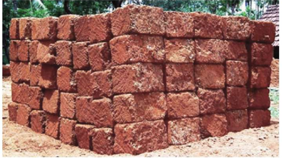
Fig.2 : Laterite, the basic building material in Goa and coastal Karnataka
