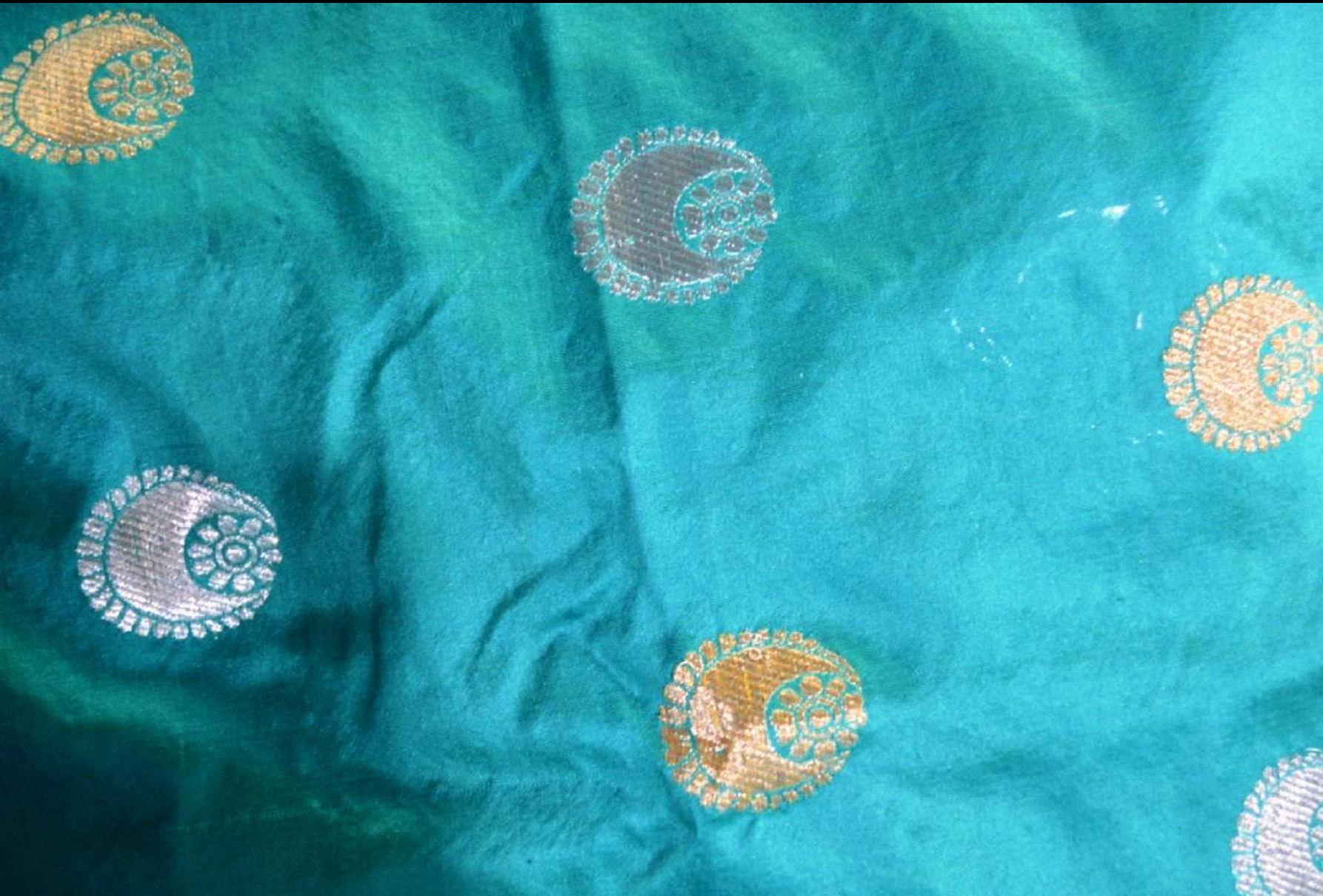
Fig.14.12 : Body of sari with Chand-tara buta ; Plain weave foundation; foundation warp and weft: silk in cyan blue extra weft: twill weave pattern in gold and silver zari
